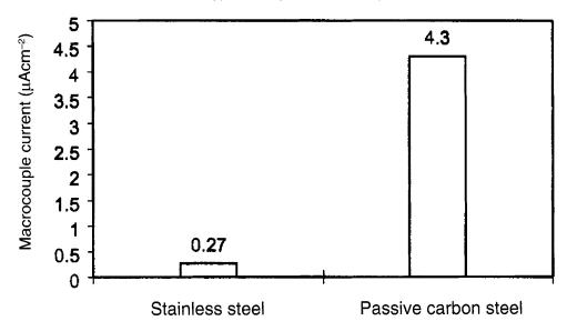
Fig. 5 Macrocouple current for stainless steel and passive carbon steel.
