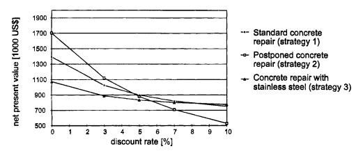
*Fig. 7* Example of the coastal bridge. Net present values (50 years remaining lifetime) for different discount rates.
